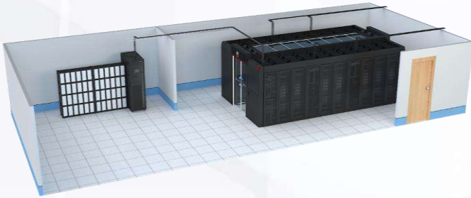
UPS Outside the Module(Integrated PDC)
